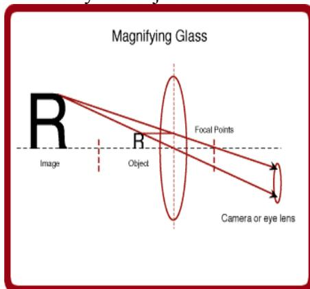
**Big idea: The objective creates a “ real image “ (can be projected on a screen) of a far away object like a star. So it “ catches” a picture of the star and bring it back to the telescope. Then the eyepiece magnifies this image for our eye. The final image is said virtual because you can't see it on a screen. The lens inside our eye projects the image on our retina.**
