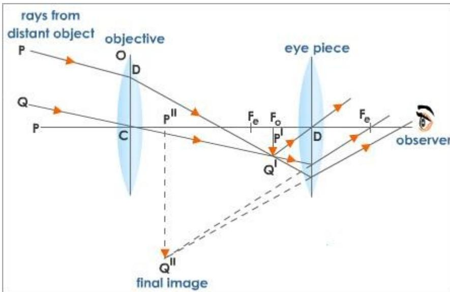
First the objective brings an image (real) of the star in the telescope. The image (P'Q') is formed in the focal plane of the objective ( $F_o$ ). Then the eyepiece magnifies P'Q' to the final image P''Q''.
