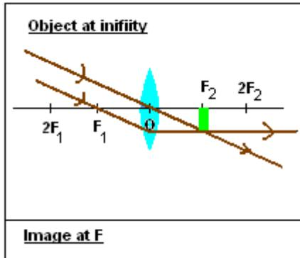
The eyepiece is a converging of short focal length used to magnify the image produced by the objective lens. See below. The eyepiece is used as magnifying glass, by means of which an enlarged virtual image is formed of an object placed just inside its focus. In this case, the object is the real image formed by the objective lens. The eye looks directly at the enlarged image produced by the eyepiece.
